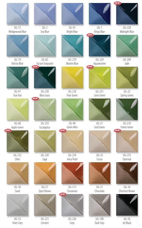
Chips shown represent Fundamentals® Underglaze applied to low-fire earthenware greenware, then fired to cone 04 bisque. Two coats of S-2101 Crystal Clear Brushing was applied to the right-side of the chip and fired to cone 06.
