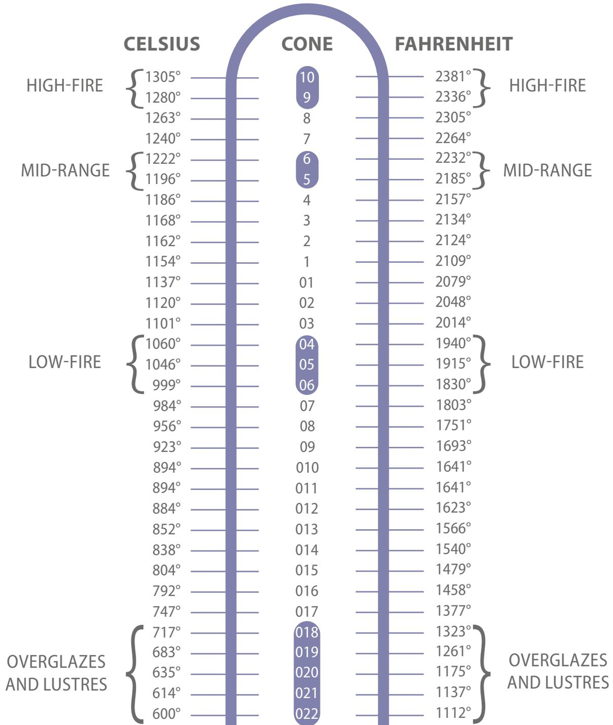
\*Cones are approximate as cones measure heat-work, which is a combination of temperature and time.
